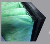
A special magnetic gasket on the Hi-Flo® ES MG allows installation of the filter without the use of fasteners or tools. The CamExtend installs as an add-on to existing HVAC built-up filter banks, giving the end user an additional 10" of filter depth. This allows facilities to capitalize on the energy savings of deep pocket, Hi-Flo<sup>®</sup> ES filters and the associated performance guarantees of that product.
