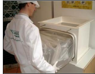
Carefully insert the filter into the housing
