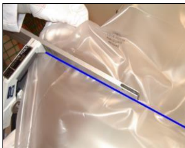
Make a first weld above the filter, sealing the bag hermetically
