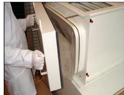
Place the door on the housing taking care not to jam the bag
