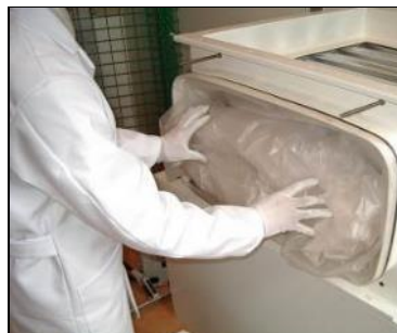
Pack the wrapped bag inside the collar
