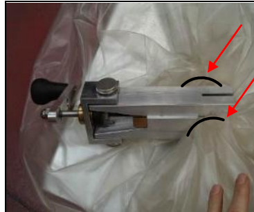
Use a cable binder on each side of the tool to help the cutting process
