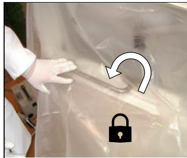
Swing the locking lever 180° all the way to lock
