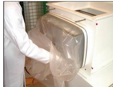
Pull the filter using the grip through the end of the bag
