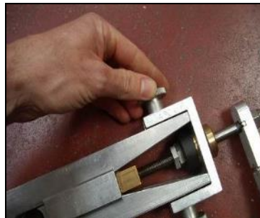
Unscrew knobs to disassemble
