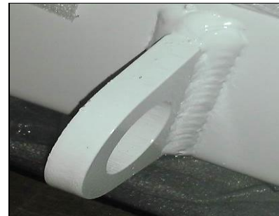
Manipulate the upper collector using the lifting rings.
