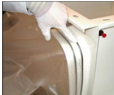
Place the O-ring of the new bag into the second groove
