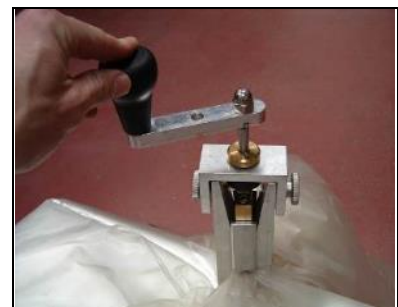
Crank the shaft to compress the bag into the U-shape
