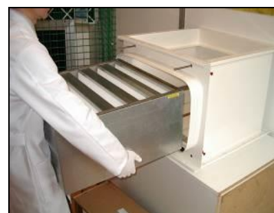
Take out the filter taking care not to touch housing sides
