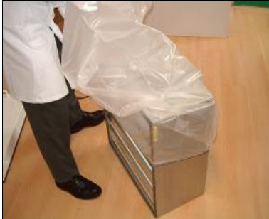
Place the filter with grip on top, slip the new service bag over it
