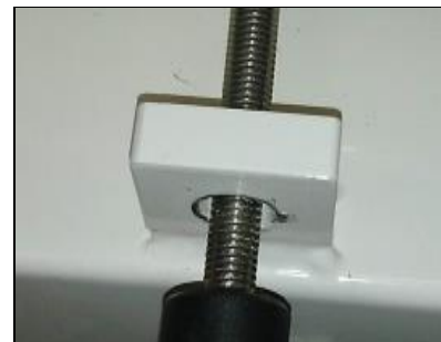
Take the door off, avoid scraping on the threaded rods
