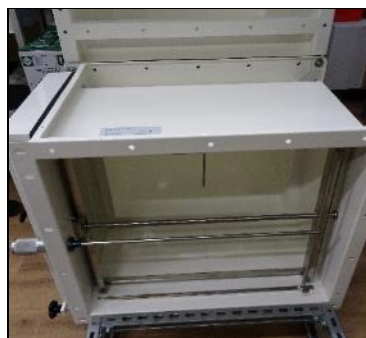
Place 1 st housing, aligning flange holes.
