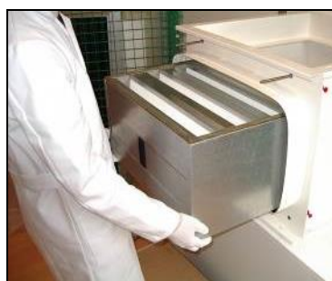
Extract the filter by pulling gently supporting the bottom
