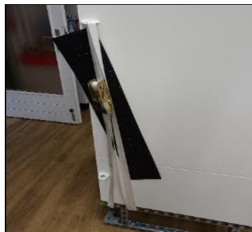
Position collector and secure against tipping over.
