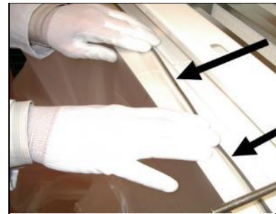
Slide the O-ring of the bag from the 2 nd into the 1 st groove of the collar
