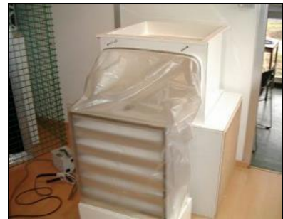
Verify correct filter orientation → Grips top & bottom
