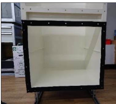
Place gasket(s) on the flange(s), aligning flange and gasket holes.
