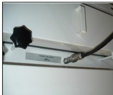
Connect Upstream Concentration Port (static)
