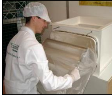
Make the bag slide over the filter while approaching the housing
