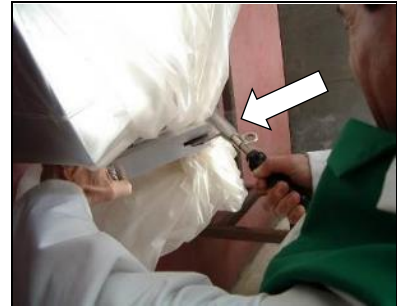
Insert the tool with a slight sawing motion until reaching the bottom of the slot
