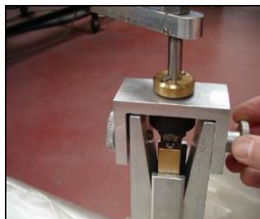
Move the mobile part to its highest position, then re-assemble
