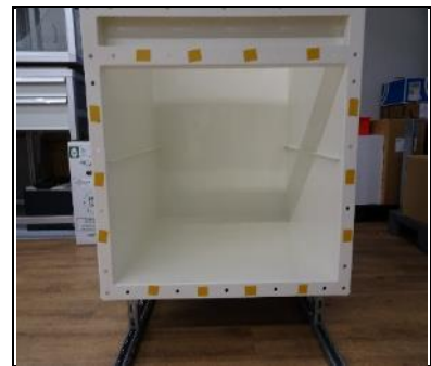
For non-adhesive gaskets, place small strips of double-sided tape on the collector flange(s).
