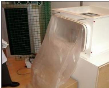
Unfold the bag - or slide the bag over the collar into the first groove
