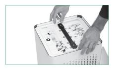
4. Take a firm grip on the pull the hatch upwards.
