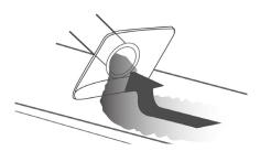
Recommended suction distance: 200 - 700 mm. The suction hood material is made from cleaning agent resistant plastic (PETG)
