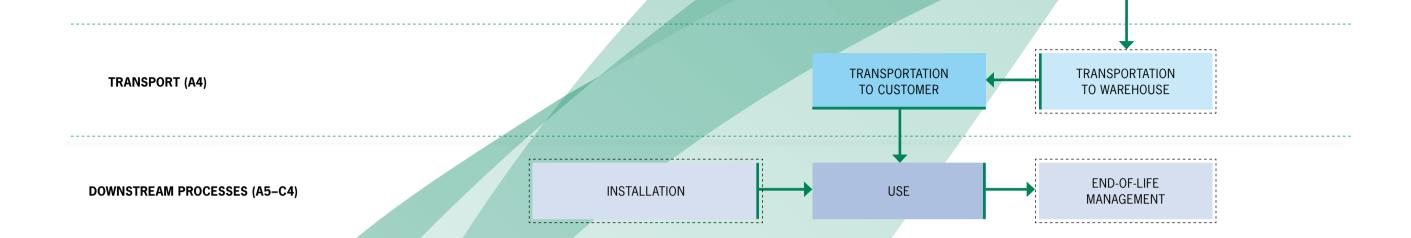
**MODULE A4** covers transportation of the filter bag to the customer. An average transport distance to the customer is assumed to be representative for the year 2019.
