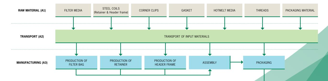
**MODULE A1** covers extraction and processing of raw materials, as well as production of the materials and components used for production of bag filters: filter media, steel coils, corner clips, gasket, hotmelt media, threads and packaging material.
