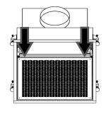
Insert new filter and slide it to the bottom
