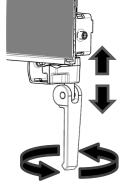
Adjust by turning the handle PU: Turn to bottom GEL: Adjust to filter height
