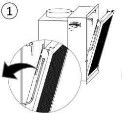
Open door and remove pressure tube from door clips
