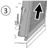
Gently slide door upwards to free hinges from slots
