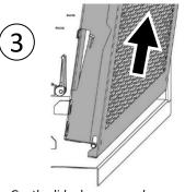
Gently slide door upwards to free hinges from slots
