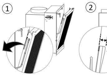
Open door and remove pressure tube from door clips
