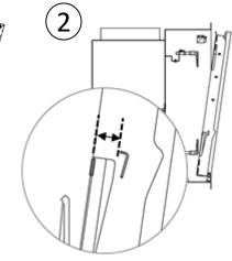
Move the door to a position where door retainers are free from Stop-brackets
