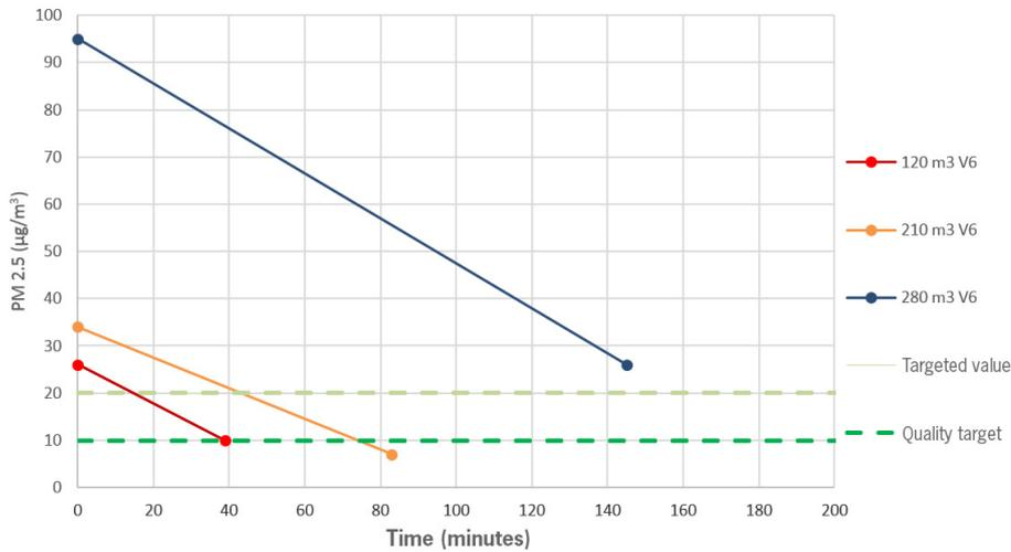
In a very polluted classroom (concentration of PM 2.5 of 25 µg/m³ and 35 µg/m³), the City M purified rooms with areas of 40 m² (120 m³) in 40 min and 70 m² (210 m³) in 85 min. It achieves the target value recommended by the WHO and even the "quality target". In the particular case of a large classroom, these thresholds were not completely met but this concerned days with pollution peak. Nonetheless, the City M enabled the IAQ to improve by 74%.
