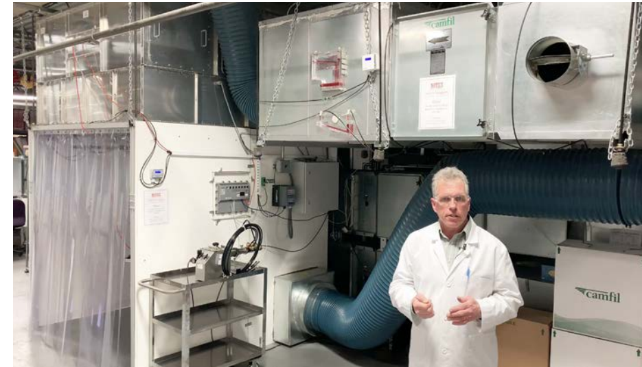
Camfil's HEPA Filter Lifetime Test Grid Riverdale, New Jersey. (Above) The grid monitors all key performance characteristics of the test filters, nine of which can be simultaneously tested not for hours or days but weeks and months, to develop a scientifically-derived predictive model. (Photo to right shows internal grid sensing system)
