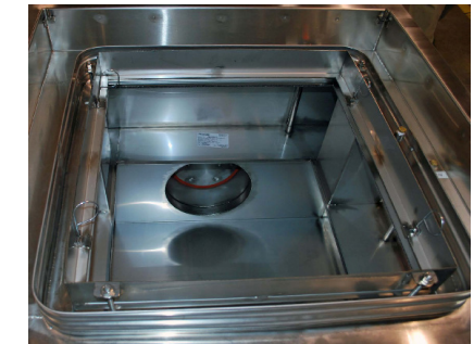
Available with an optional slip flange, the HEPA filter may be removed within an enclosed bag for the protection of service personnel and convenient removal of contaminated filter.
