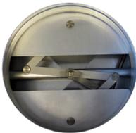
**Guillotine Damper** - This damper facilitates room balancing and airflow control. It is easily adjusted using the 1/4-turn rotary mechanism attached to a robust mechanical linkage and heavy-duty blades. The damper assembly is welded to the hood body to increase rigidity and eliminates "binding" of damper blades common in pop-riveted units.
