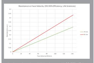
The above chart shows initial resistance with 99.99% efficiency Megalam EnerGuard, panel, for resistance values for other efficiencies please contact factory. The Camfil Megalam EnerGuard Ducted Ceiling Module (DCM) is ideal for applications where clean air is a requirement to protect products, people, and the environment. The Camfil Megalam EnerGuard DCM includes:
