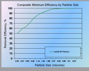
The efficiency chart above is extrapolated from particle size versus efficiency information when evaluated per ASHRAE Standard 52.2.
