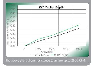
The Cam-Flo XLT bag filter combines the strength of a multi-layered, polypropylene media with a reinforced, rigid ABS frame to create a robust air filter that is strong enough for even the most extreme conditions. It has been tested in laboratory conditions to a static pressure exceeding 33.0"w.g. (equivalent to 172 pounds per square foot). It is ideal for turbulent or high pressure applications where normal HVAC filters would fail.
