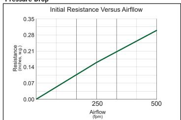
(Schedule air filters for change when initial pressure drop has doubled.) Final pressure drop should not exceed 1.5" w.g.
