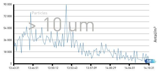
A peak in the graph shows when welding begins and how quickly CamCleaner remove these particles.
