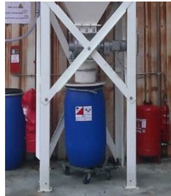
Discharge adapted to the quantity and type of dust collected
