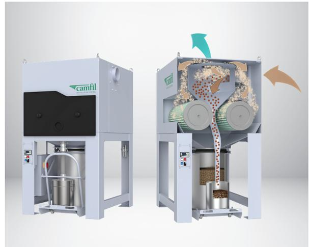
Compact dust collector QS2 from the Quantum Series, specifically designed for extraction of single laser tables. Units available in three different sizes with air volumes from 1,500 up to 5,500 m<sup>3</sup>/h.
