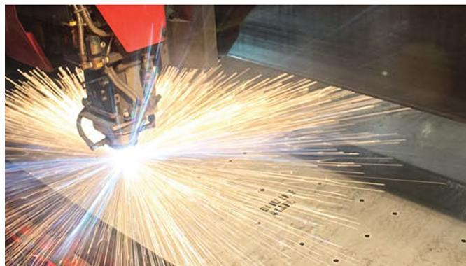
A Camfil APC promotional part is produced on a 4 KW laser table.
