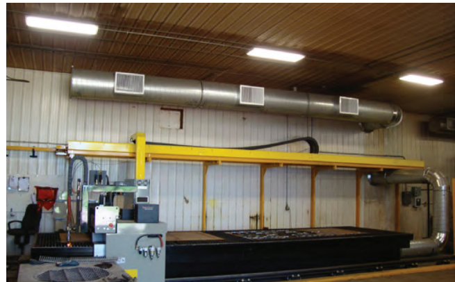
Example of a dry downdraft table: Contaminants are exhausted to an outdoor dry media dust collector that captures dust and fumes.
