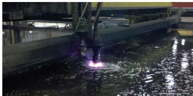
Plasma cutting on a water table creates a dirty, high-maintenance environment.
