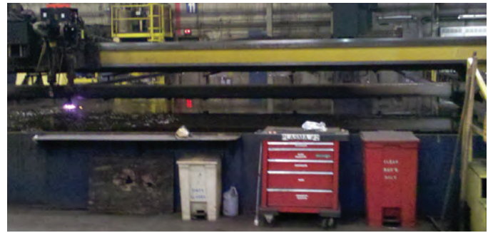
Example of a wet plasma cutting table designed to contain the majority of dust and fumes as parts are cut in the water.
