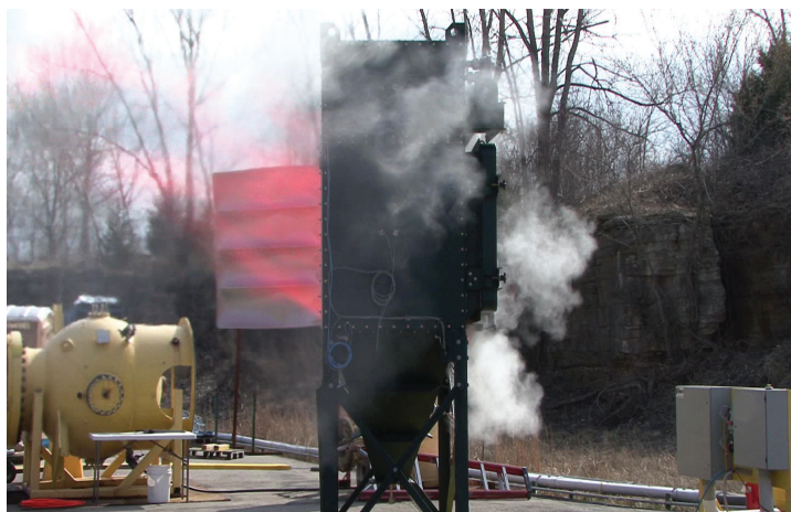
Staged explosion is performed to test whether a dust collector explosion vent will work as intended. The vent has popped open to relieve internal combustion pressure, keeping the collector from blowing up in a combustible dust explosion.
