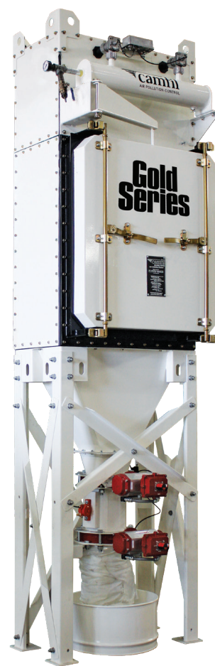
Dust collector for tablet press application is readied for installation. It contains two high-efficiency filter cartridges, bag-in/bag-out safe-change filter system and safe-change continuous liner discharge using an explosion vent on the back of the collector.
