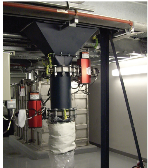
Continuous liner discharge system contains dust released from the cartridges to the hopper during automatic pulse cleaning of a dust collector.
