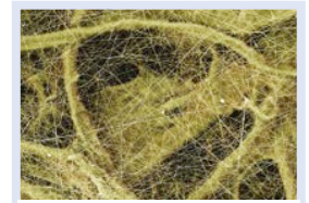
Filter media with nanofiber coating
