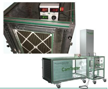
During a CamTester filter test, the airflow can be adjusted to duplicate the test unit's CFM or to a flow rate commonly used for comparative purposes. The pressure drop in inches of water gauge is displayed as well as the watts required to power the fan. The CamTester information reveals the filter with the lowest total cost of ownership.
