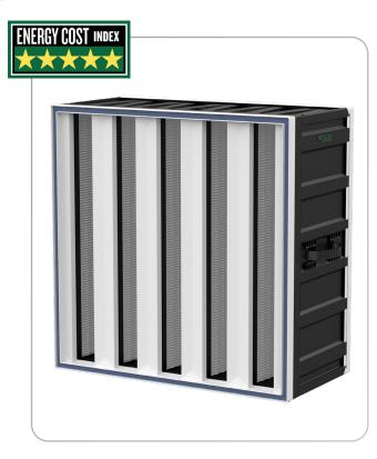
The Camfil Absolute VG Gel seal filter provides high-efficiency particulate air (HEPA) filtration for critical application processes in the pharmaceutical, microelectronics, healthcare, semiconductor, and other industries. Its media surface area, more than twice that of standard HEPA filters, provides an optimal combination of high airflow capacity and low resistance to airflow. The Camfil Absolute VG Gel seal filter offers:
