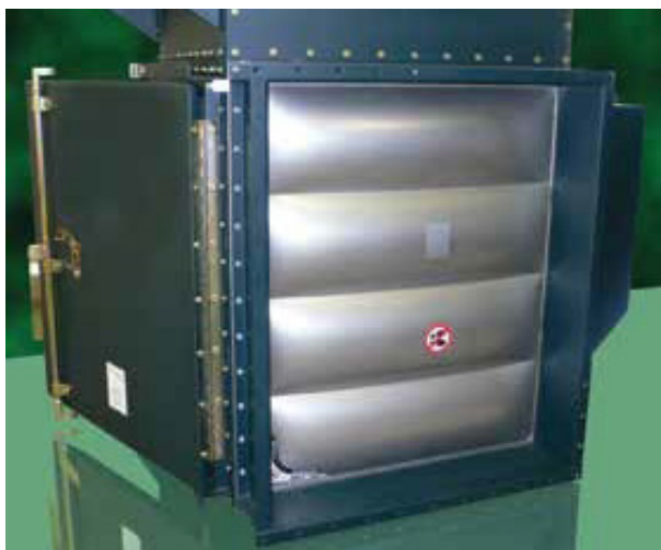
Designed to be the “weak” link of the vessel, explosion vents open when pre-determined pressures are reached inside the dust extractor allowing the over-pressure and flame fronts to exit to a safe area. Explosion vents minimize damage to the dust extractor caused by overpressure created by a deflagration.
