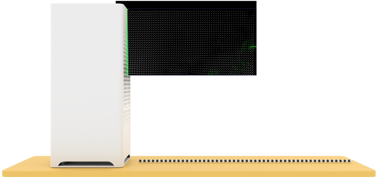
FIGURE 7. PIV measurement for the inflow to the City-M with an aerosol generator placed 1m to the right. Shown is the velocity field overlaid on a single video frame. Note also the 1m scale bar.
