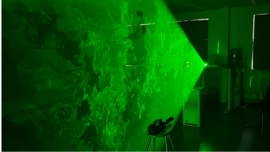
FIGURE 5. Photograph depicting the test setup used for measurements at the Camfil site. Note the laser expanded laser sheet in green, the aerosol generator in the foreground and the large amount of aerosol used to seed the flow. The City-M is observed below the laser source.
