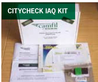
Citycheck IAQ kit sensors can be used to sample common indoor sourced contaminant concentrations that can be a risk to health. The two main types test for are volatile organic compounds (VOC's) and Aldehydes.
