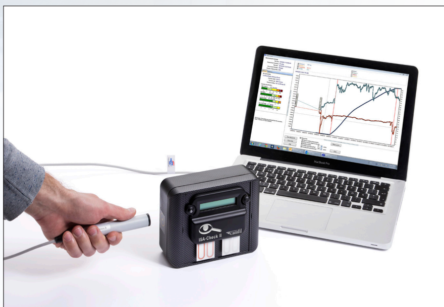
ISA-Check II unit with data pencil and laptop based software.
