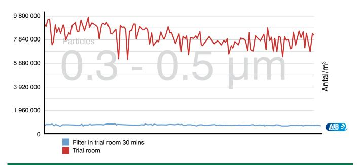
THIS CHART SHOWS CAMCLEANER MAKES A SIGNIFICANT REDUCTION OF PARTICLES IN THE OFFICE SPACE ON THE WASTE SITE. AS WELL AS THE REDUCTION IN PARTICULATE, THE USE OF ACTIVATED CARBON FILTERS MEANT STAFF REPORTED LESS FOUL SMELLS MIGRATING FROM THE RECYCLING AREA INTO THE OFFICES.
